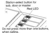
To call a TB-SE sub, the other master or audio door station pick up handset and depress a station-select button. When called by tremolo tone, pick up and depress the LED-lit select button. LED remains on while in communication. Communicating TB-M is notified of a call with a lit LED only. The audible call tone will resume when the handset is hung up.
